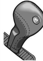
To select Sport mode, press the "S" button on the selector lever when the selector lever is in position N or D.
